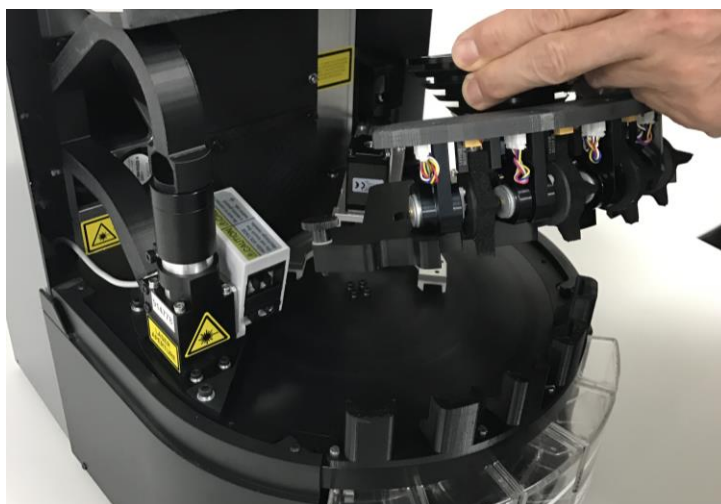
Figure 25 - Lifting the Stone Guide Plate
