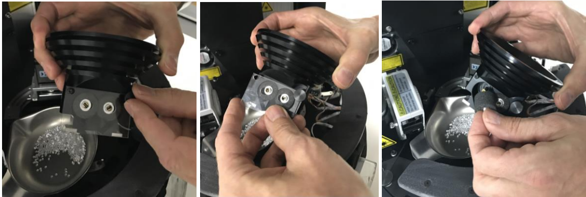
Figure 22 - Removing Hopper Rollers
