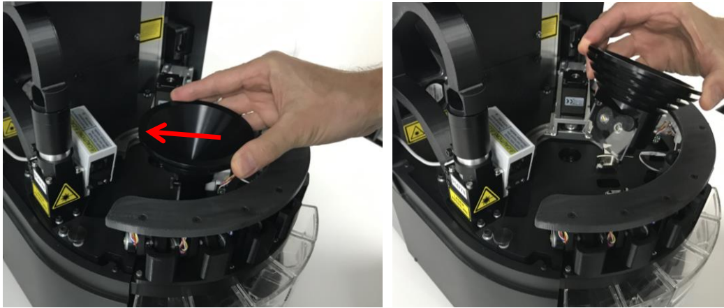
Figure 21 - Removing the Hopper
