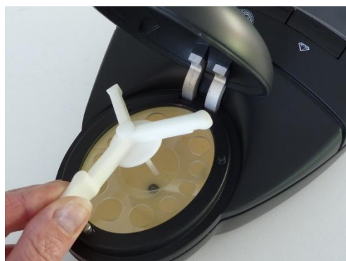
Figure 3: Locating the sample holder into the sample chamber
