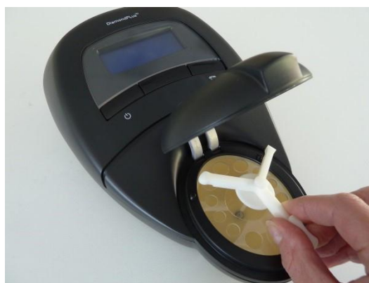
Figure 1: Placing a stone into the sample chamber
