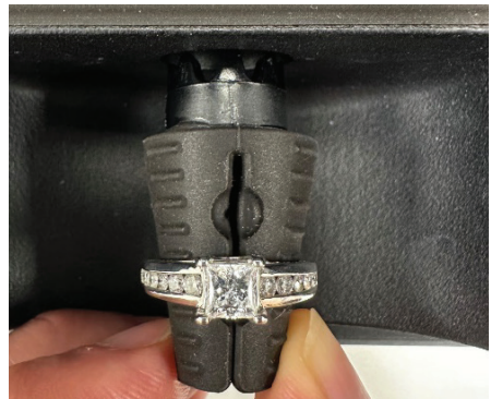
Figure 8 - Positioning the cone
