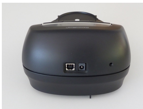
Figure 3: Power socket location
