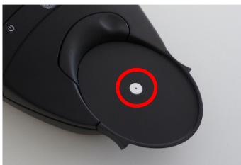
Figure 14 White fibre ferrule situated in the centre of the sample dish.
