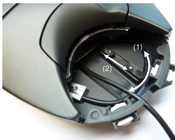
Figure 22: Re-assembling the fibre cable
