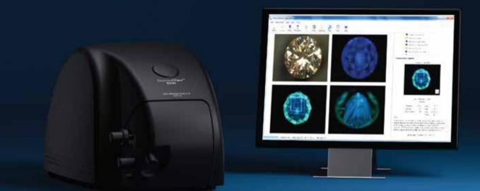
DiamondView Zoom features an UltraXGA USB 3.0 camera with 60% higher resolution than the previous DiamondView. This enables the operator to analyse images on a wide range of diamond sizes, from 0.01 ct to 10 cts, using a single instrument.
